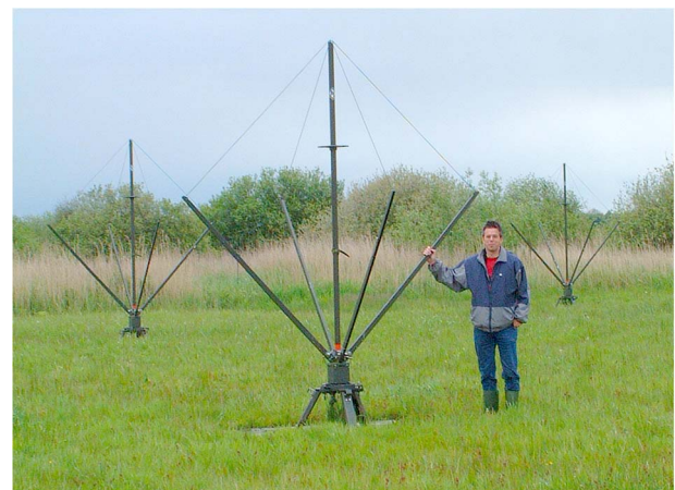
Figure 8. Three of the nine crossed-loop antennas of the R&S DDF0xM RDF.
