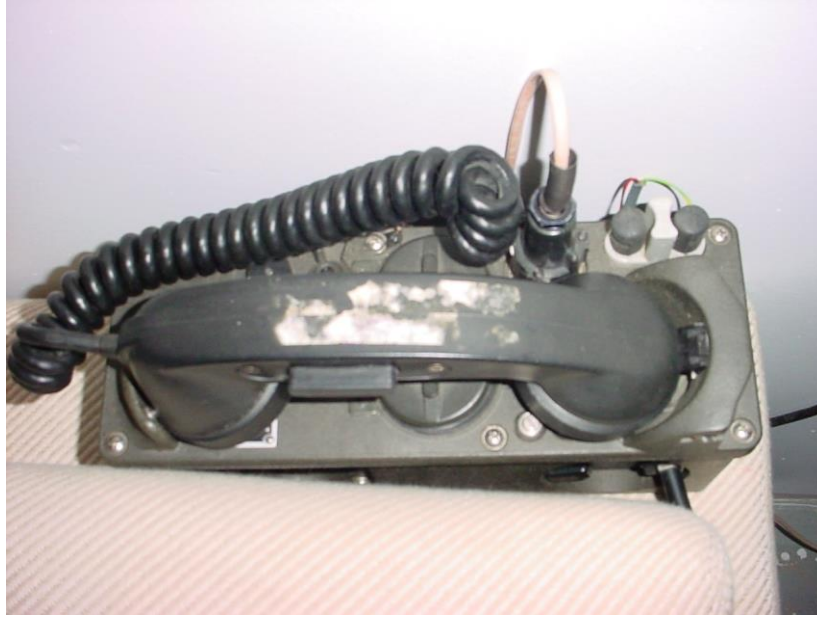
TA-312 field phone. Notice plug coming out of top of phone. This goes to the phone patch.
